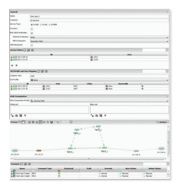
The system allows definition of multiple types of providerdefined SLA profiles which can include CIR, EIR, CBS, and EBS for each level. Profiles may also include advanced hierarchical quality of service where the DSCP values and CIR limits can also be set for the real time applications like voice and video and how the remaining bandwidth can be allocated between the business critical and best effort applications.
