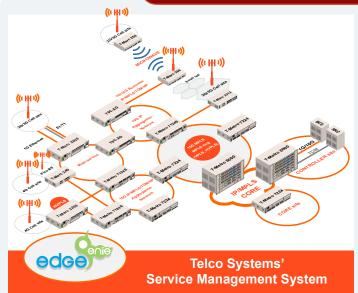
Our solution supports all legacy 2G and 3G networks and is optimized to meet the new HSPA+, WiMAX and LTE networks requirements including support for multiple technologies co-located at the cell site.
